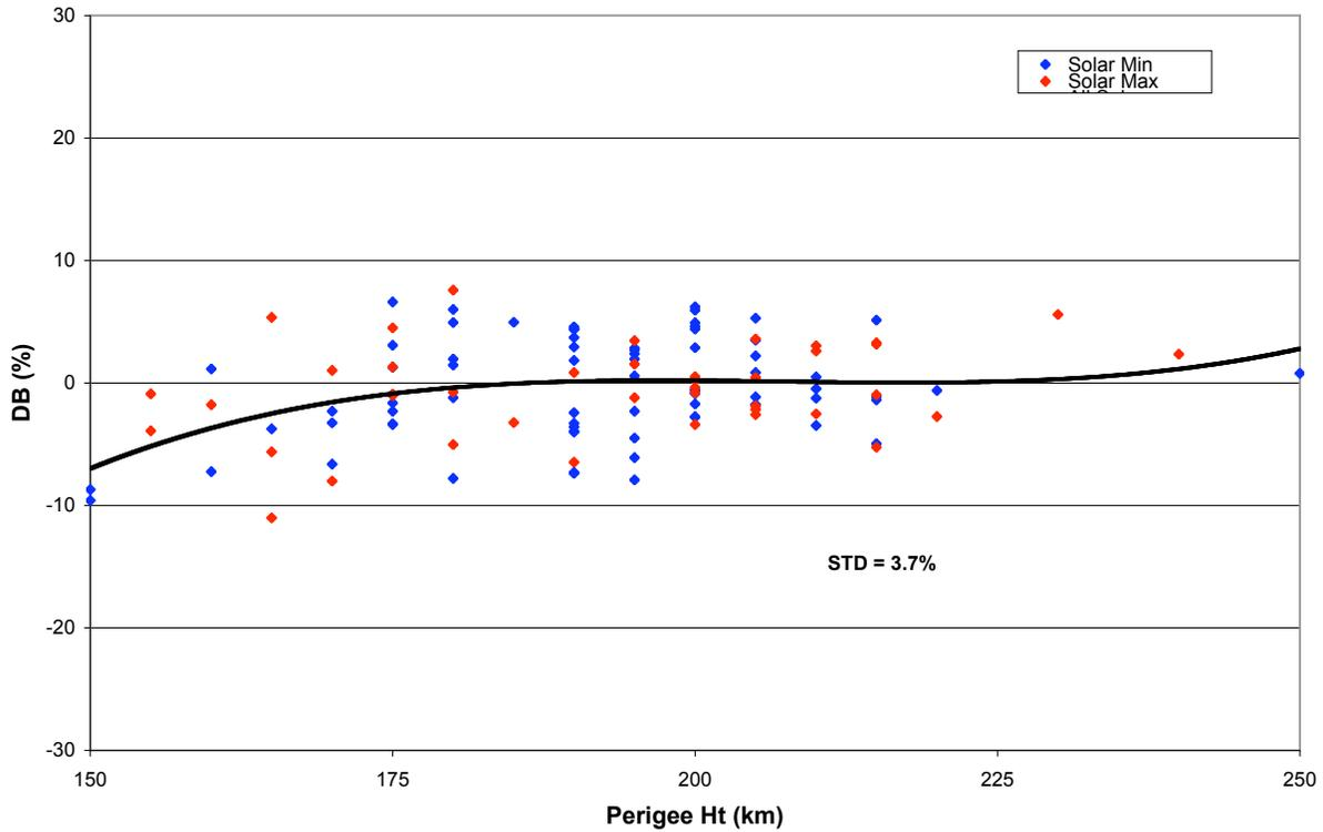
Figure 1. Delta B (average yearly values) for PAM-D rocket bodies are plotted as a function of perigee altitude. Values for solar maximum and solar minimum years are separated by color.
