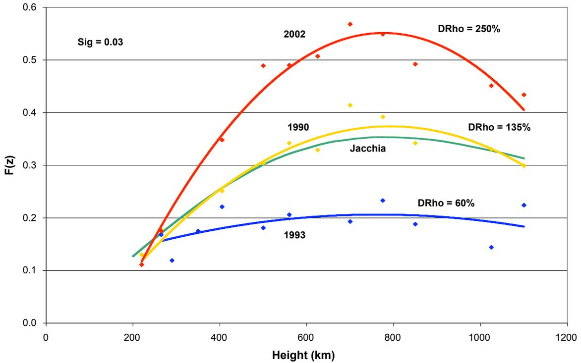
Figure 2. The amplitude function  $F(z)$  for three different years (1990, 1993, 2002), with semiannual amplitudes plotted for each satellite for each year. The standard deviation, 'sig', of the fits is shown. The constant  $F(z)$  function from Jacchia is also plotted.
