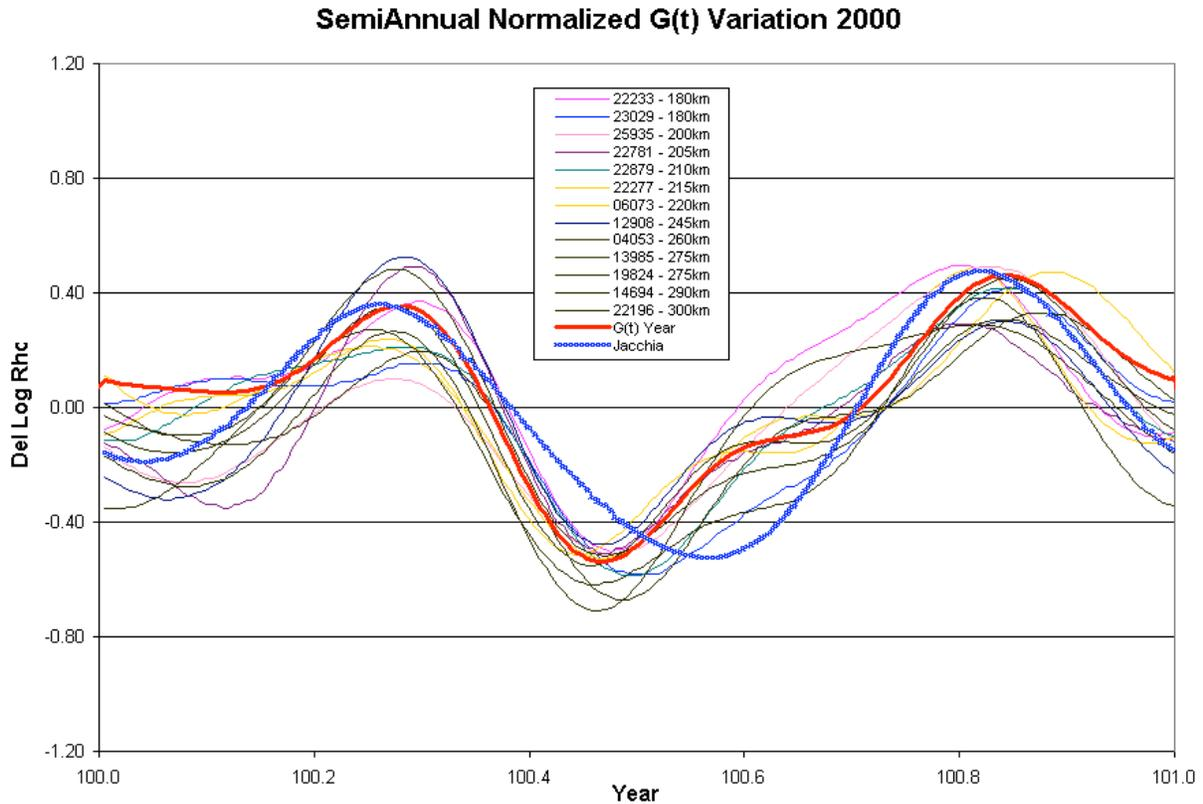
Figure 6. The low altitude individual satellite G(t) fits are plotted for year 2000. The Jacchia model and the yearly fit model are also shown.
