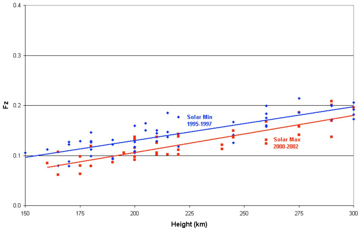
Figure 3. The semiannual amplitude function  $F(z)$  is plotted for solar minimum (1995-1997) and solar maximum (2000-2002) years as a function of height.
